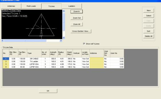
In this window the tower elevation is shown along with the tower cross-section at the bottom of the Tx-line. To add a new line or group of lines select **New** and a blank line with a line type (none) is shown. The user inputs the following data as defined below:
