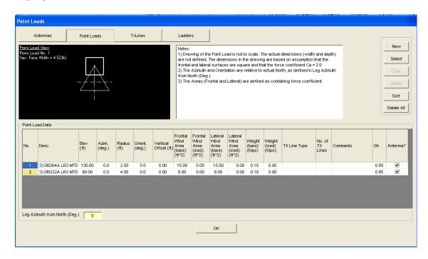
In this window the tower elevation is shown along with the plan cross-section at the point load elevation. To add a new point load select **New** and input line with zero values is shown. The user inputs the following data as defined below:
