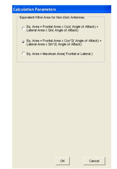
For non-dish antennas, the user can select the calculation method for the equivalent wind area of non-symmetric antennas.
